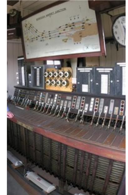
Above – A composite shot of the frame with the lower cover off, showing the interlocking bars. This miniature frame was an important intermediate step between the old mechanical frames and electrical push-button types
