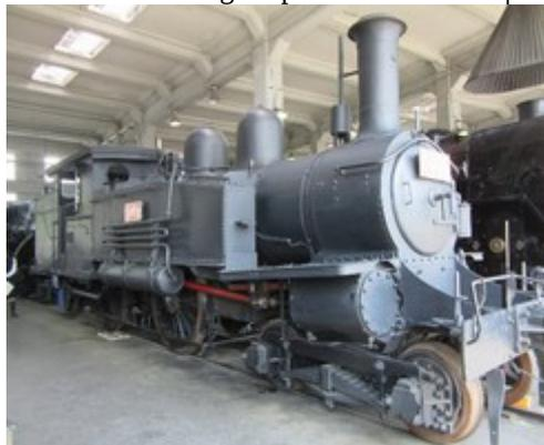
British built loco No 1080 of D9 class, 1901. Mainly used for hauling mineral trains on private lines.
