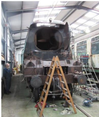
**34051 at Ropley in August:** the smokebox front has now been further stripped down and undercoated, together with the buffer beam, tender side sheets and footplate.
