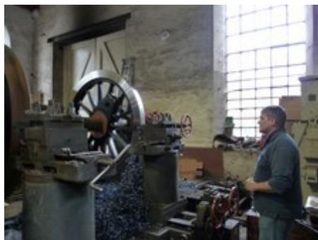
Jeff Phelps demonstrates the wheel lathe at the Flour Mill
