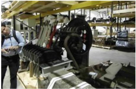
Rack of signal levers, superheater header, and stone signs.
